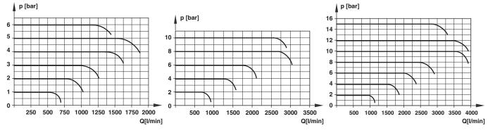
Flow rate characteristics NG 16/connection plate 1/2" (NG12); P1=7 bar, 12 bar, 17 bar
